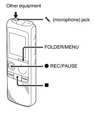
You can make music files without using the computer by recording the sound from other equipment connected to the IC recorder.
